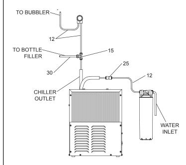
Figure 3 - LZWS-LRPB Tube Routing
