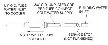
Figure 12 – Water Supply Connections
