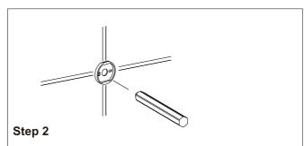
Position the backing plate flat side down on the wall and mark holes with pencil.
