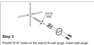
Predrill 3/16" holes on the wall to fit wall plugs. Insert wall plugs into the wall. Position backing plate flat side down over the plugs and install screws.
