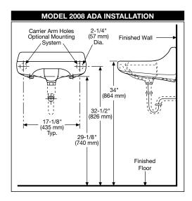
— 8" (203mm) 3-1/2" (89 mm) (102 mm) 4" (102 mm) 3-1/2" (210 mm) (89 mm) 18-3/4 10-3/4 1-3/4" / (44 mm) Dia. (273 mm) Leveling and locking screw holes for concealed arm 16" (406 mm) (533 mm) Finished Wall 5/16" (8mm) Dia Anchor Holes Mounting Bracket 3" (76 mm) 10-1/4" (260 mm) 34" (864 mm) 33-1/2" (775 mm) 3/8" (10 mm) Dia. S.P.S. Supplies of slot in 32-1/2" (826 mm) 1-1/4" (32 mm) Dia. O.D. W aste To center wall stringe 26" (660 mm) Finished 23' Floor (584 mm)
