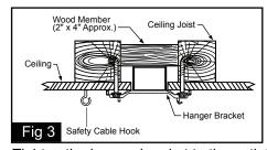
Tighten the hanger bracket to the outlet box with two mounting screws.
