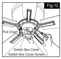
Make sure the wires of the fan light in the switch box are capped with wire connector. Secure the switch box cover into switch box with the switch box cover screws.
