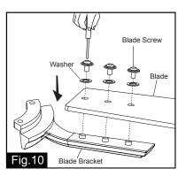
Mount each blade bracket to fan blade using three blade screws and washers.
