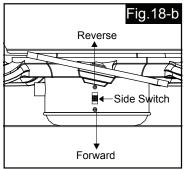
The slide switch on switch box sets direction of fan rotation. Select the desired direction of fan rotation.
