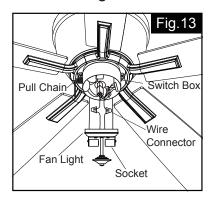
Remove screws from fan light first, then connect the white (neutral) wire from the fan light to white (neutral) wire from switch box with a wire connector, connect the black (hot) wire from fan light to blue (hot) wire from switch box with a wire connector.
