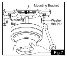
Attach the mounting bar to mounting bracket with metal washers and hex nut by hand and then free your hands to secure the hex nut by spanner.
