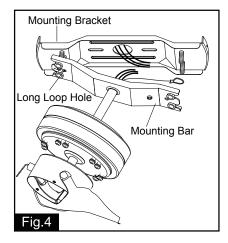
Unscrew hang motor assembly onto mounting bracket. Insert the long loop hole of mounting bar to the poth hook for hands-free wiring. (See Fig.4)
