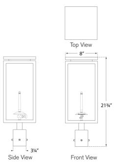
Gas light fixture supplied with 3/16" copper gas line and 3/16" x 1/4" gas line adaptor
