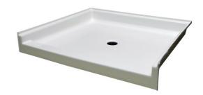
Warm Rain model B 4038 shower base fixtures are constructed of reinforced polyester resin covered with a high gloss gel-coat of 18 - 20 mil. thickness. The reinforced fiberglass has a minimum content of 18 % fiberglass.
