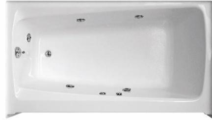
Warm Rain model WR 610WP (right hand plumbing) and WR 611WP (left hand plumbing) whirlpool tubs are constructed of reinforced polyester resin covered with a high gloss gel-coat of 18 - 20 mil. thickness. The reinforced fiberglass has a minimum content of 18 % fiberglass.
